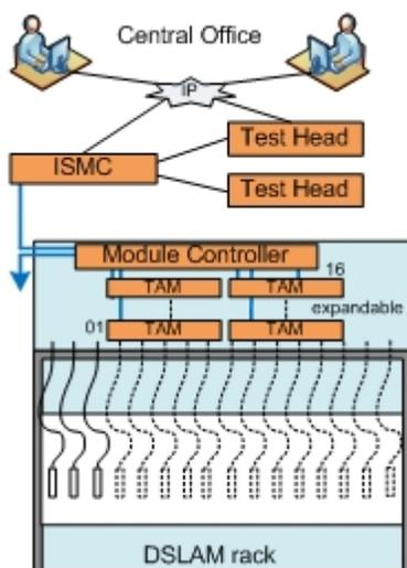
The DSLAM cable is connected to the DSLAM side of the module and a tie cable fitted to the other side and returned to the DSLAM. Retrofit takes less than an hour, the cables are removed from the Module, the modular TAM replaced and the cables re-connected. The installation teams will be provided with all the tools required to carry out a retrofit installation.
